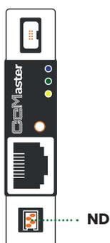
**Figura 11:** Detalle conector negro del bus principal
